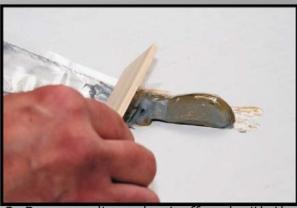
Remove clip and cut-off end with the clear material and apply entire contents to mixing surface; ensure mixing surface is not porous.
